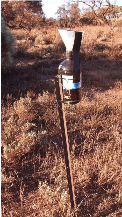
Figure 19: Bottle type dust trap – landholders stated this type of device should have been used by Arrium on their but was not, despite being used elsewhere around the mine and at Iron Baron mine.
