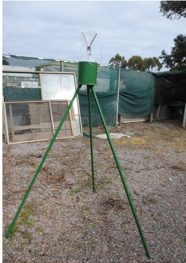
Figure 20: A commercially available dust deposition gauge as per Australian Standard, claimed by landholders to be the type of dust monitoring device Arrium should have installed on their properties
